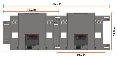
The wall-mount bracket allows 16-inch battery-to-battery spacing:
