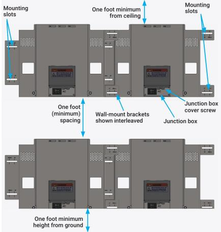
e. Verify that the wall-mount bracket is solidly attached to the wall.
